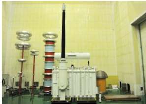
The world's first DFP-410000/1000 generating transformer developed by TBEA is used in China Power International's Anhui Pingwei 2×1000MW supercritical generating unit.
